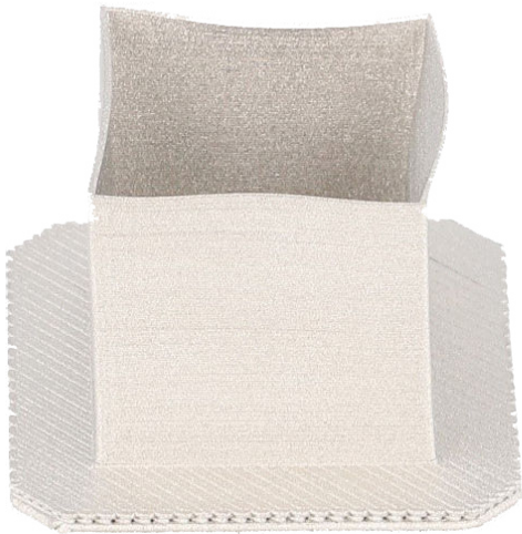
Figure 12. 0,4 mm Wall Failure
