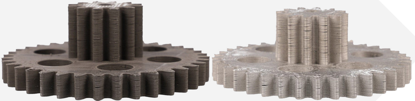
Figure 20. Print Delamination become sintered cracks
