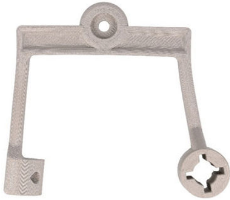
Figure 21. Part with distortions after D&S
