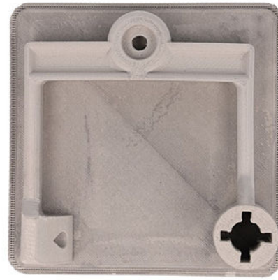
Figure 22. Use of shrinkage plate ensure uniform shrinkage
