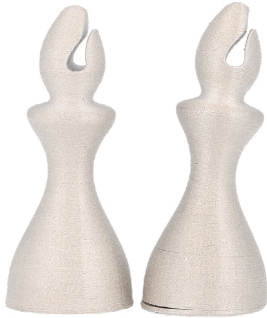
Figure 16. Warped Bottom can lead to failure
