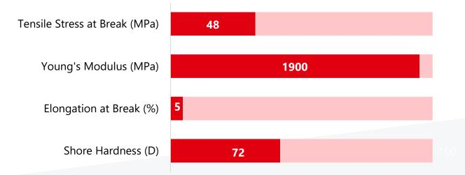
\*Values shown are linked to parts printed on a DLP printer at 385nm & post cured with broad spectra bulb (Loctite UVALOC 1000)
