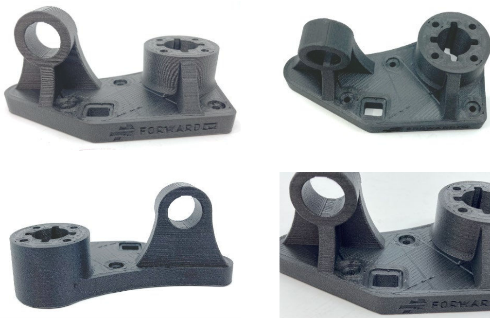
Figure 3. Printed object where the used filament had a moisture content of \geq 0.07 w%.
