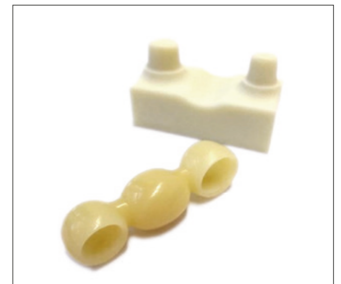
Fig. 8: Test specimen geometry for the chewing simulation
