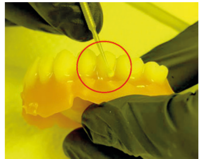
Fig. 17: Removal of the excess with a brush
