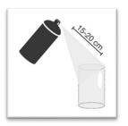
Apply AESUB transparent from 15-20 cm away. Gently push down the spray button and move the can across the area using even, back and forth strokes. Move at a consistent pace to achieve an even coating. Spray over the entire
