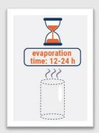
The applied layer of AESUB orange evaporates independently after scanning. The otherwise time-consuming cleaning after application is no longer necessary.
